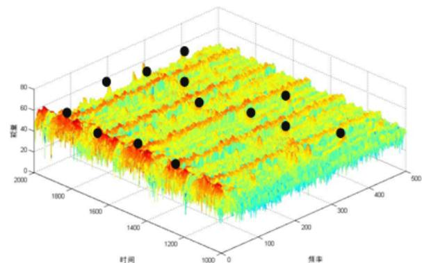
Figure 2. Spectrogram with Highlighting Energy Peaks[1]
