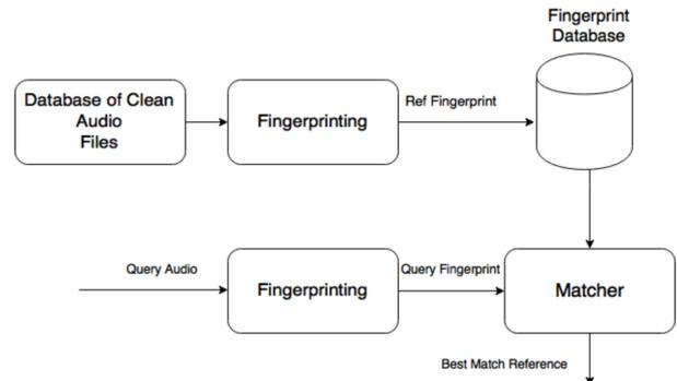
Figure 1. Generalized Audio Fingerprinting System
